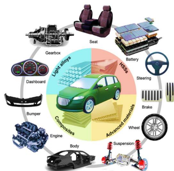
Figure 2 The most common lightweight materials utilised in vehicle components are light alloys [16]
