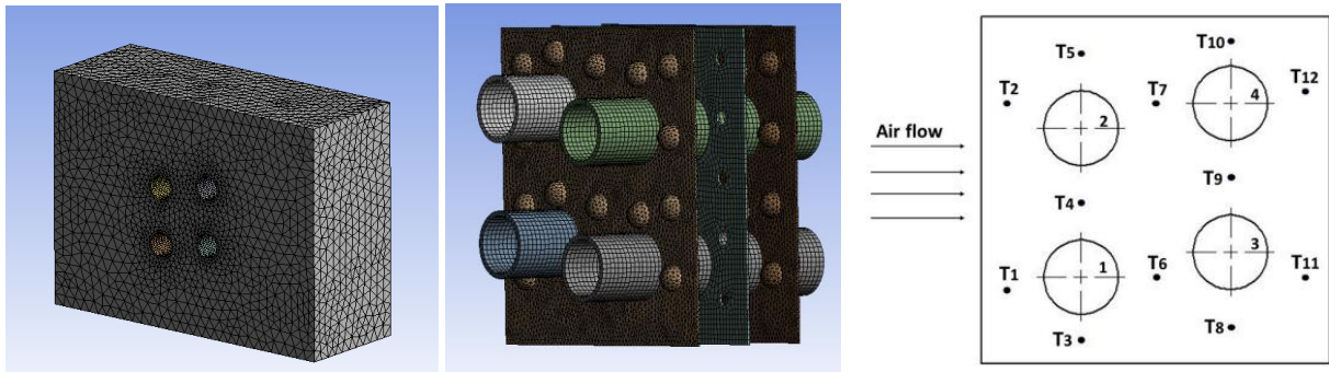
Figure 4 Mesh generation of computational domain and notation of tube
