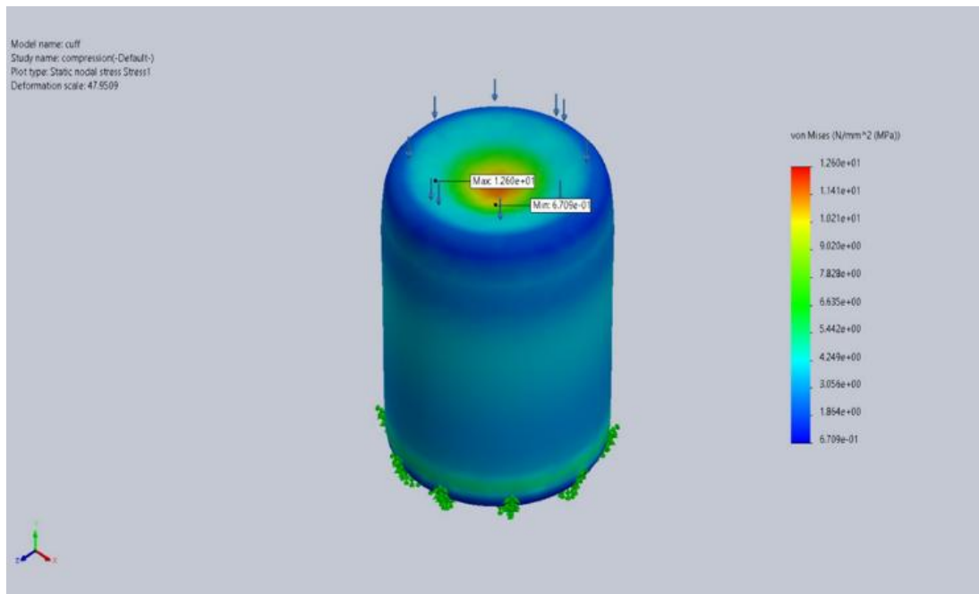
Figure 3. Mechanical Compression Stress Analysis for Endoscopic Gastroscope Tip Jackets [PLA Based tip-3(a), PEEK based Tip-3(b)]
