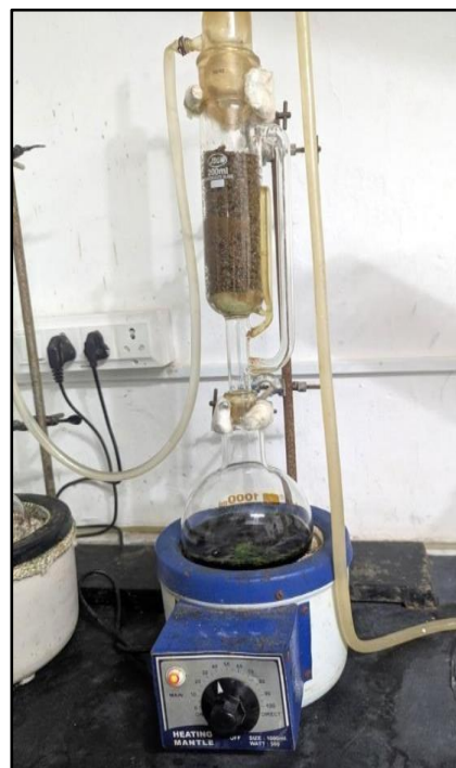
Figure 2: Soxhlation process of plant extract by methanol & petroleum ether
